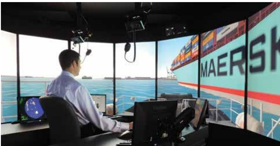
The view from the helm of a MITAGS 300-degree tug bridge simulator.
