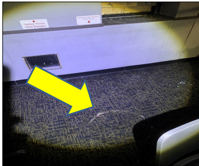
Figure 3: Escape hatch (yellow arrow).
